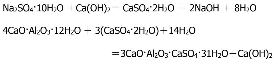
The volume of product AFt is 1.5 times larger than the volume of substances before the reaction. This forms great internal stresses within the concrete structure resulting in the expansion and contraction of the concrete, and over time, the structures strength will be lost. This can be considered a kind of chronic and stubborn disease to concrete.
