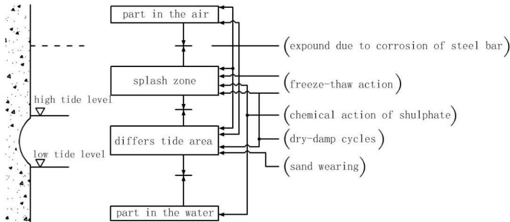
Fig 1 different positions suffer different corrosion for the reinforced concrete structure under marine environment
